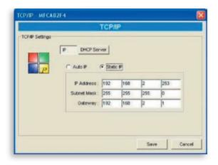
The Print Server will check if the manually configured IP address is in the same subnet as the network or connected computer. If the TCP/IP-address settings configured manually are in a different IP subnet than that of the connected networking devices, the user will be prompted by the alert message shown below. Click "OK" to go back and configure the correct IP-address settings for the Print Server.
